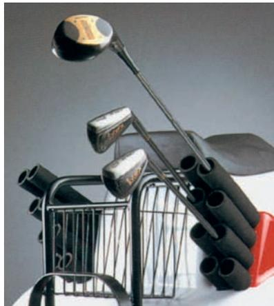
*Conceived for golf courses, this electric three-wheel battery-operated vehicle, protected by an international patent and produced by a company founded for this purpose, serves various functions, and may be used both as a golf cart to transport one person, or as a cart to carry golf clubs during competition, compatibly with the rules of golf. A fundamental element is the handlebar, which is articulated to be extendable and swung down so that it may be pulled from behind at walking speed.*
